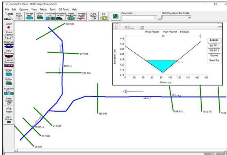
**Figure 21: Cross Section and Water Surface Profile on River Stream in Sub-Basin 1.**
