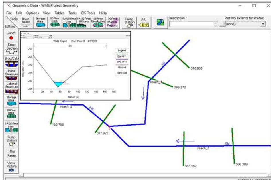
**Figure 22: Cross Section and Water Surface Profile on River Stream in Sub-Basin 2.**
