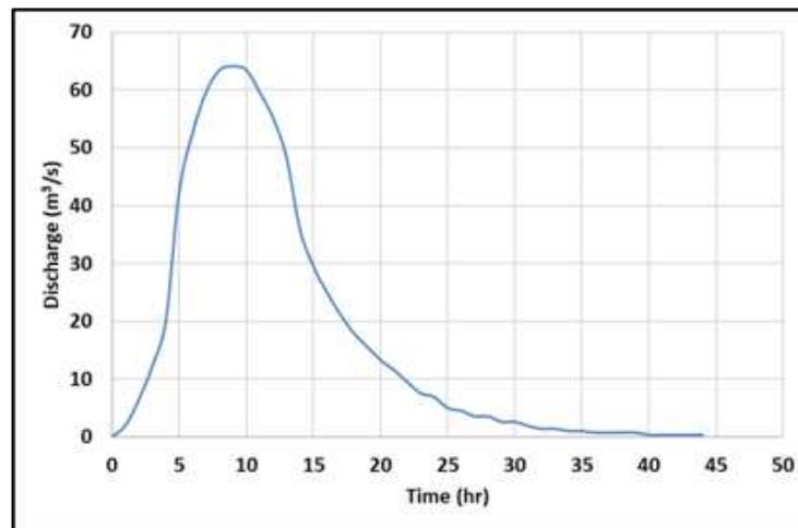
**Figure 18: Unit Hydrograph for Zarqa Ma'in Catchment Area.**
