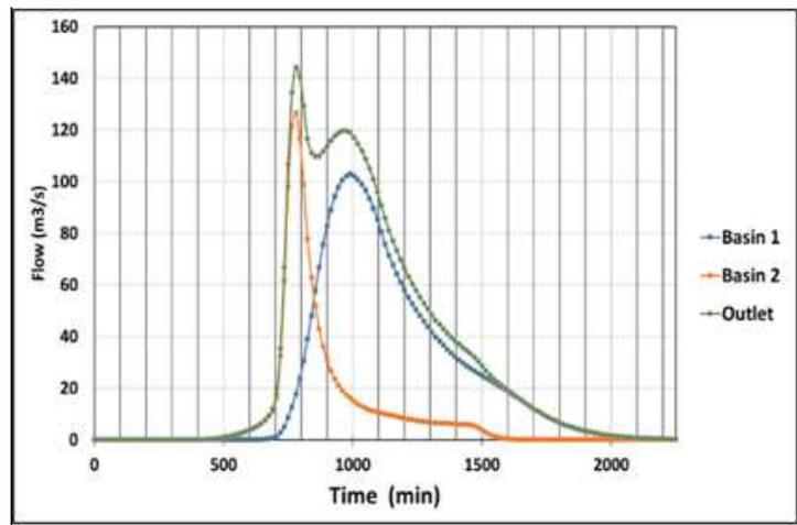
**Figure 20: Peak Flow Discharge Hydrograph Created by WMS (11.0) for the Two Sub-Basins and at the Outlet.**
