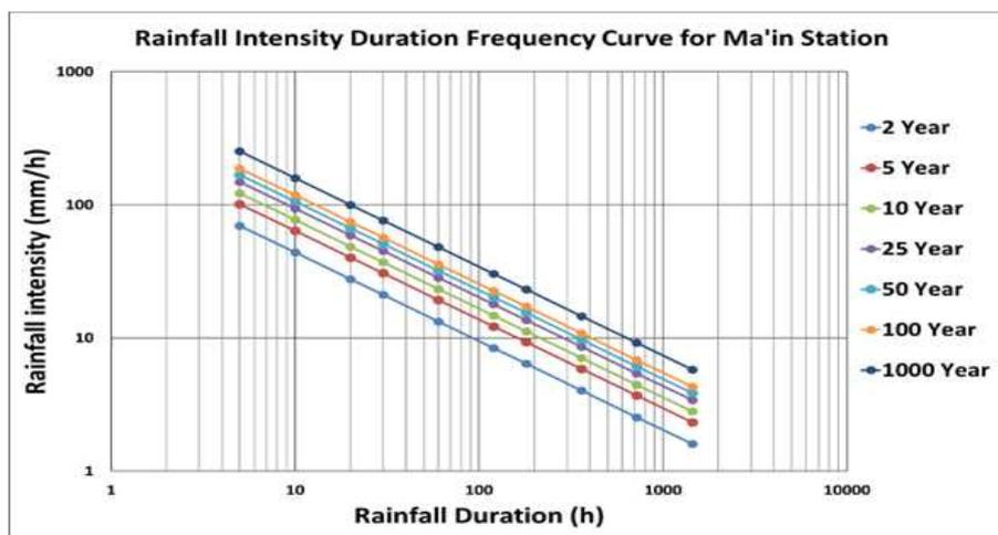
**Figure 15: Intensity-Duration-Frequency (IDF) Curve for Ma'in Rainfall Station.**
