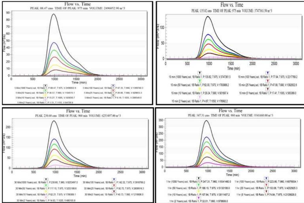
**Figure 17: The 5, 10, 30 and 60-Minute Hydrograph of the Different Return Periods for Zarqa Ma'in Catchment.**
