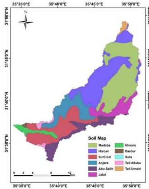
Figure 6: Soil Types of the Zarqa Ma'in Catchment Area (HTS and SSLRC, 1993).
