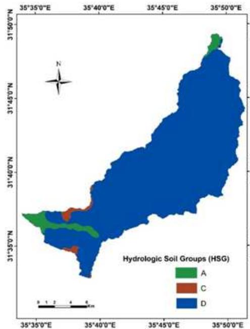
Figure 7: Hydrologic Soil Group in the Zarqa Ma'in Catchment Area.
